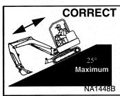
Never exceed 25° when going down or backing up a slope.
