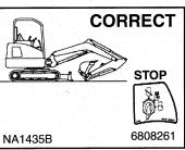
To leave excavator, lower the work equipment and the blade to the ground. Stop the engine.
